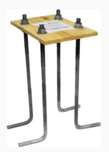
Strong Poles' pre-engineered Anchor Baskets makes installations much faster, and alignment much easier. Simply push the Anchor Basket down into the wet concrete until the template is flush with the top of the concrete, and be sure that the conduit rises well above the hole in the template. Then before the concrete is cured, Remove the template and make sure foundation is level and smooth to mount the pole.
